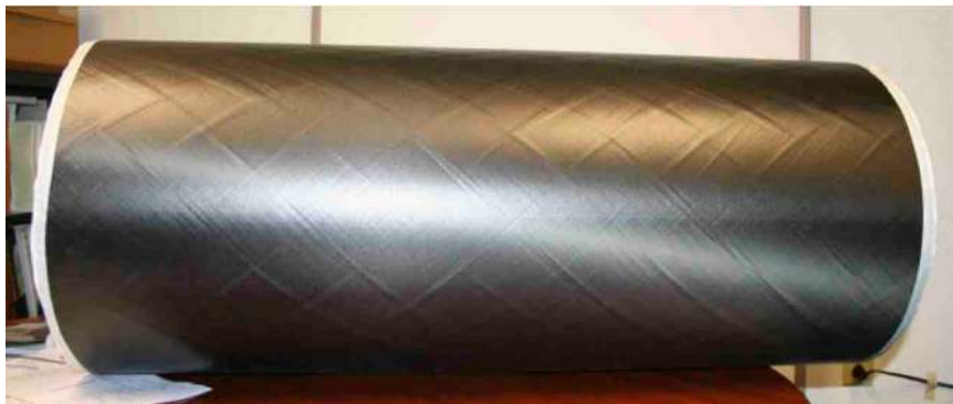
Figure 2. Advanced composite tow-steered shell
