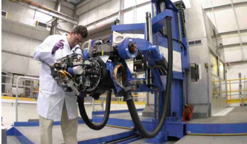
Figure 1. Fiber placement system (Lockheed Martin)
