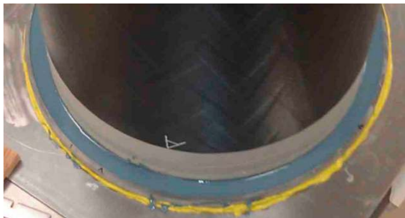
Figure 7. Potted end of tow-steered shell
