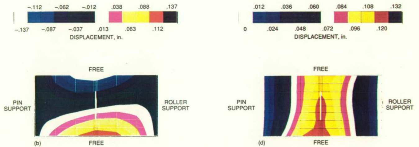
Figure 14.—Mode shape fringes after 91 percent loading. Fracture load, 6086 lb; support condition 1.
