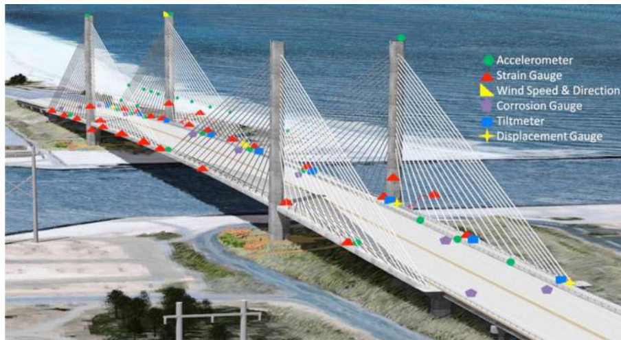
FIGURE 1 | Layout of sensors in the SHM system.
