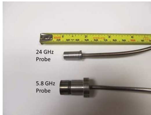
Figure 1. – Microwave blade tip clearance probes (Meggitt).
