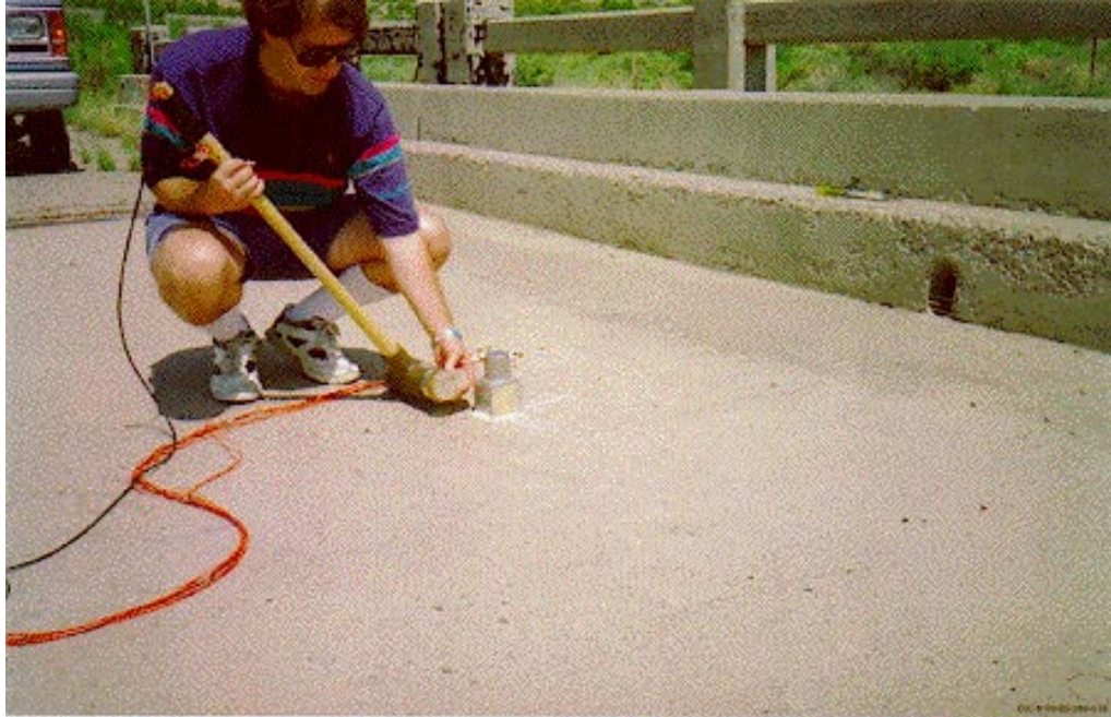
Figure 19. The hammer and accelerometer used for the impact test.
