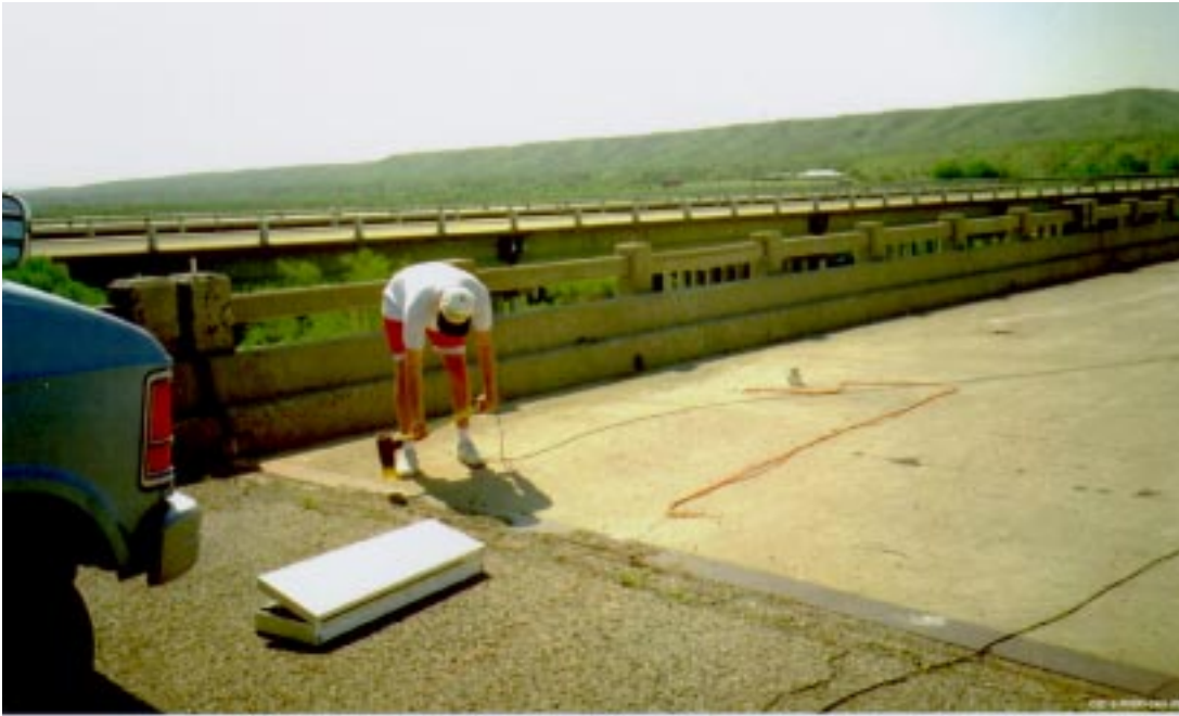
Figure 21. An impact being applied to position 2.
