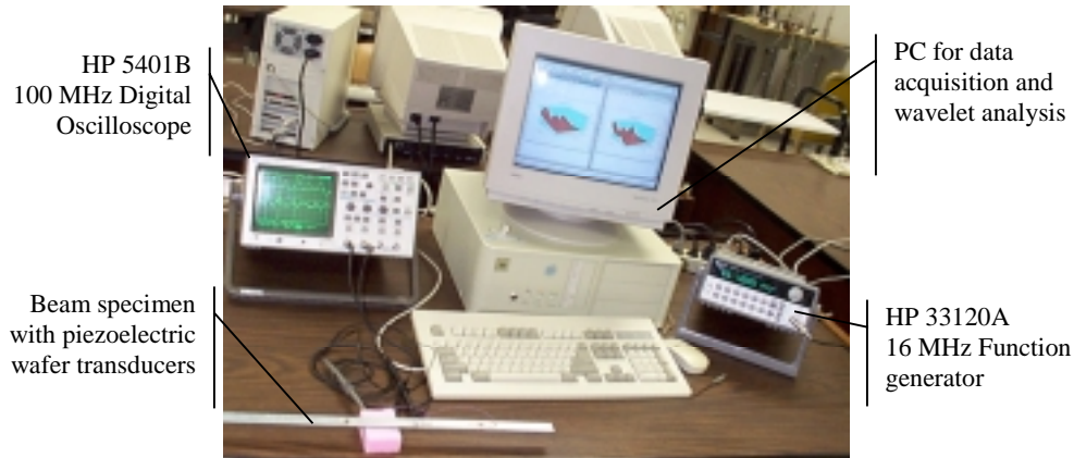
Fig. 1 Experimental setup for beam impact tests with piezoelectric wafer transducers and wavelet transforms.
