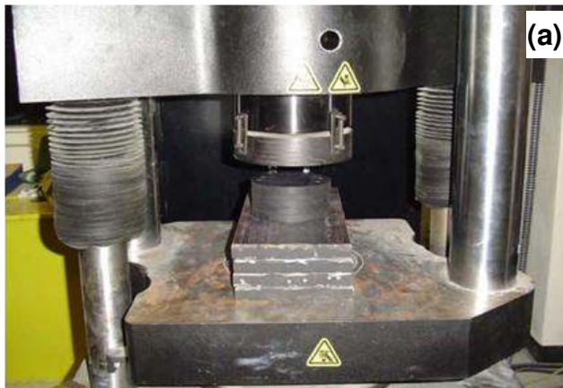
Figure 48: Compression tests of duro-50 pads using a universal testing machine (a) and spring constants at the anticipated support reaction interval (b)
