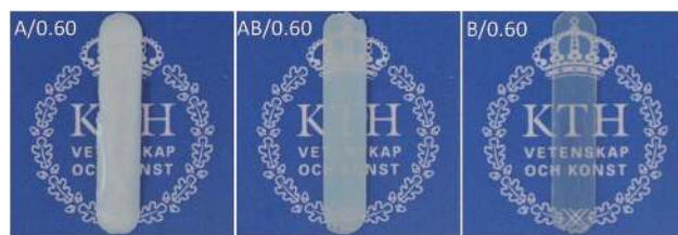
Fig. 3 Visual appearance of samples A/0.60, AB/0.60 and B/0.60. Typical appearance of samples used in the DMA and EIS measurements.
