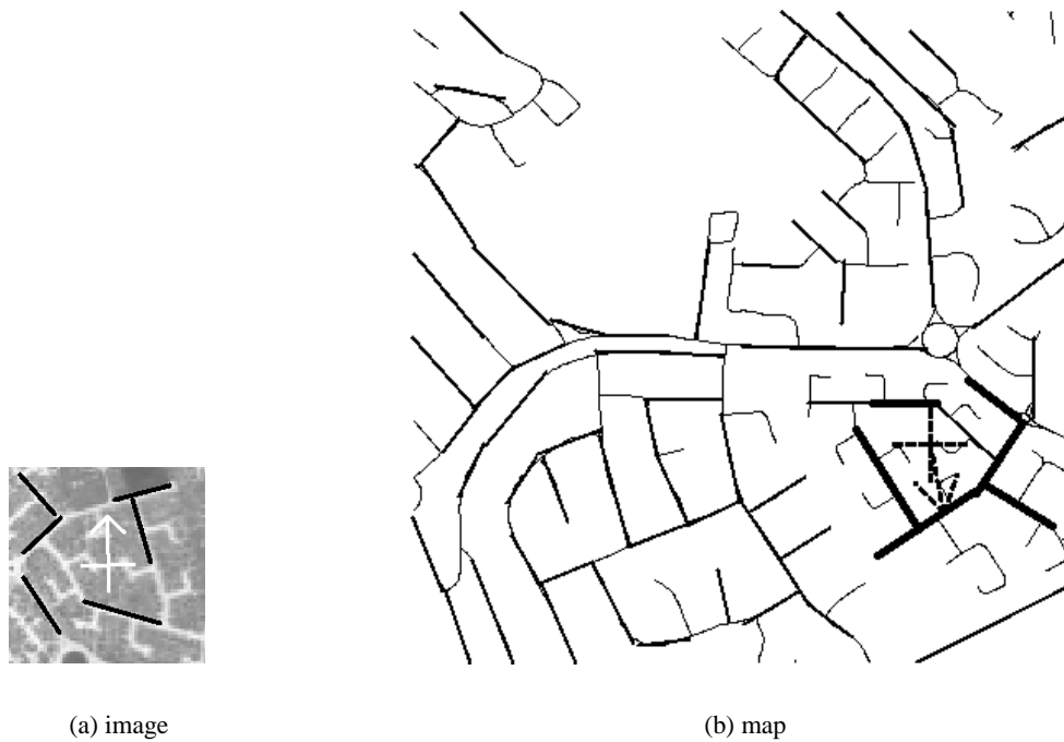
Figure 7.4: Correspondences after the 1st pass, showing the computed relative position and orientation
