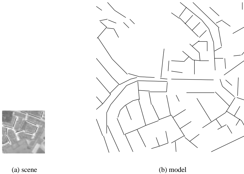
Figure 1.2: Scene and corresponding model with extracted line segment features
