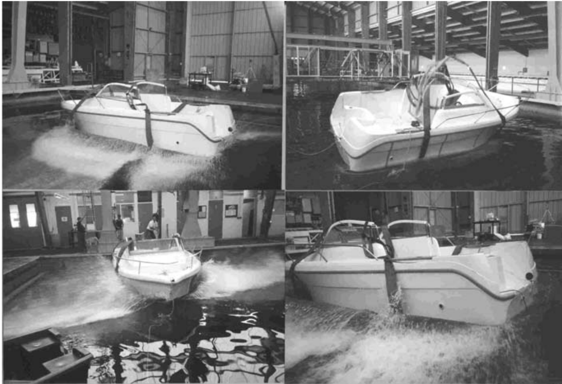
Fig. 7 Photos showing boat drop tests
