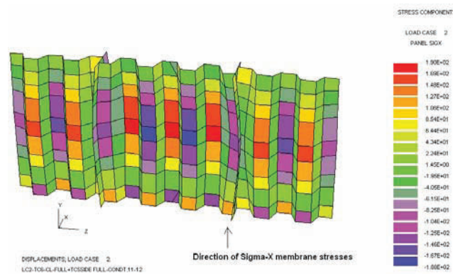
Figure 9 Prototype analysis – VC version - LC2 - \sigma_x membrane stresses (N/mm 2 ) Slika 9 Analiza prototipa – VC verzija - LC2 - \sigma_x membranska naprezanja (N/mm 2 )
