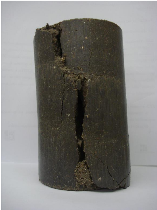
Figure 8: Triaxial failure mode of mixture M1 (consolidation stresses of \sigma'_{v0} = 150 kPa and \sigma'_{H0} = 75 kPa)
