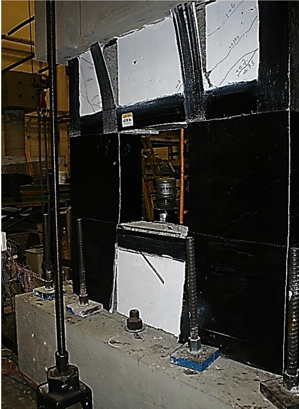
Figure (13): Failure of Wall Specimen (R-WO)
