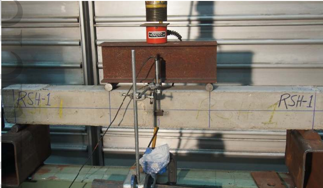
Figure 3: Experimental setup for four-point loading
