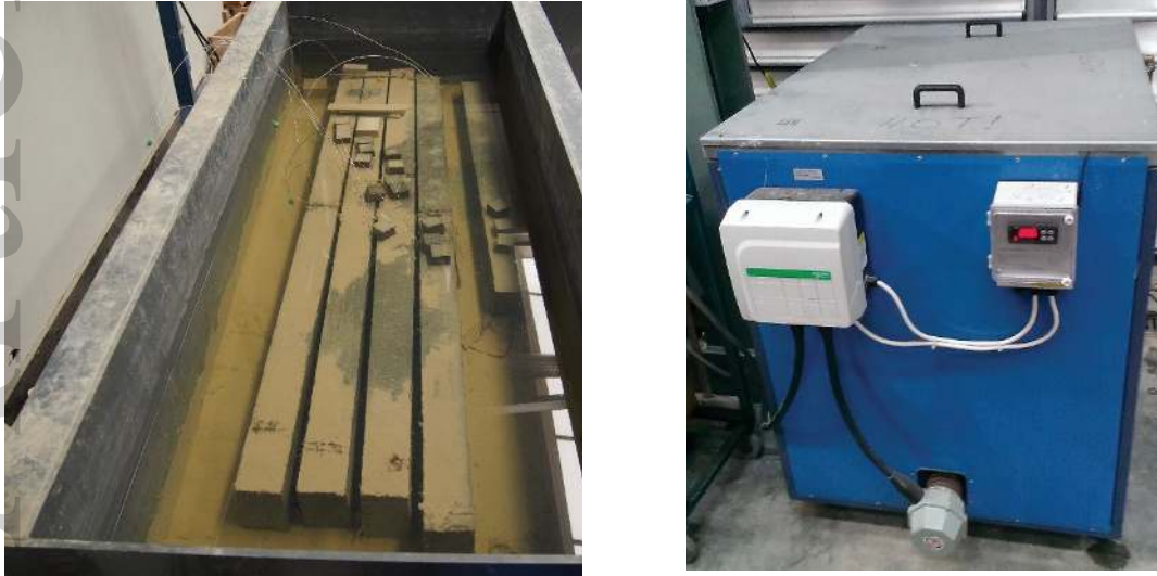
Figure 2. Left) cold curing tank, right) hot curing tank
