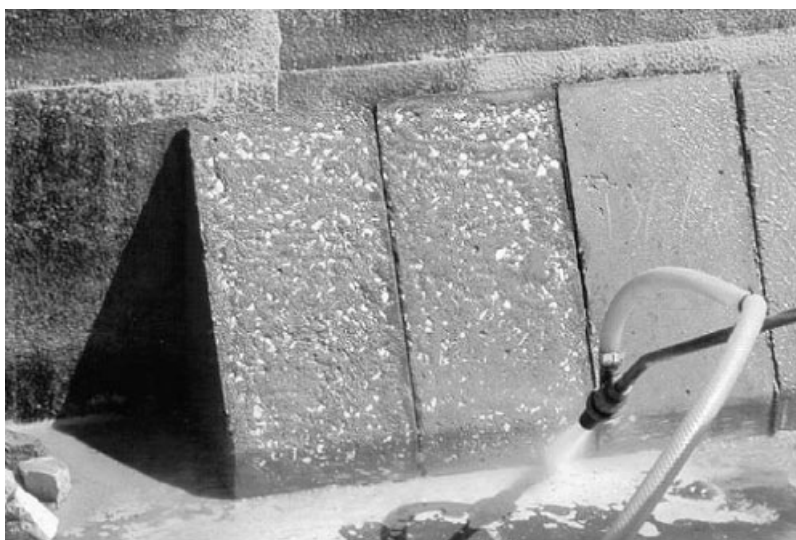
Fig. 3 Slant shear specimens prepared by sand-blasting
