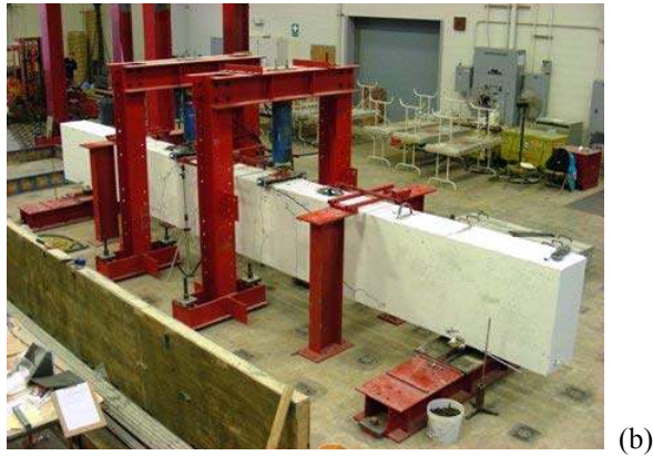
Fig. 4. Test setup for Specimens 1, 2 and 3A: schematic (a), and photograph (b).
