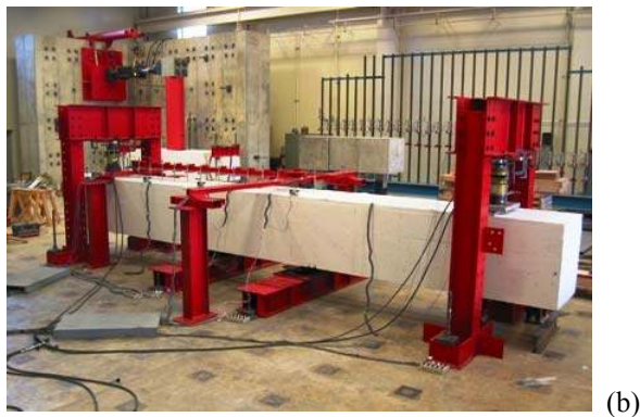
Fig. 5. Test setup for Specimens 3B and 4: schematic (a), and photograph (b).
