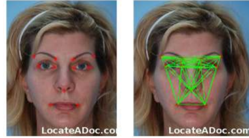
Figure 9. The 11 landmarks and the 83 triangles for the calculation of the triangle descriptor.
