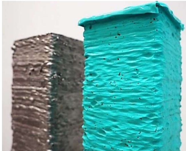
Figure 10: Silicone replica of the inner surface profile of typical SHS specimens
