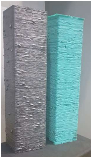
Figure 10: Silicone replica of the inner surface profile of typical SHS specimens
