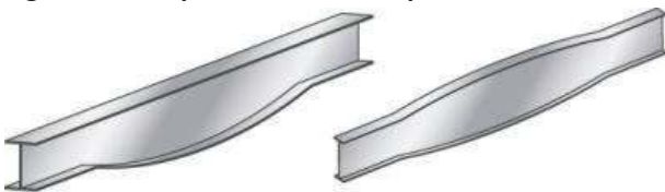
Figure 6. Examples of Variable Depth Beams.
