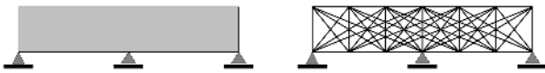
Fig. 3. Modelling of a beam as a solid continuum and a truss-like structure.
