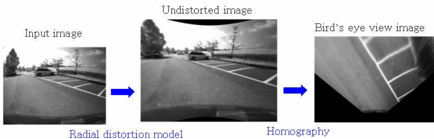
Fig. 2. Construction procedure of bird's eye view image
