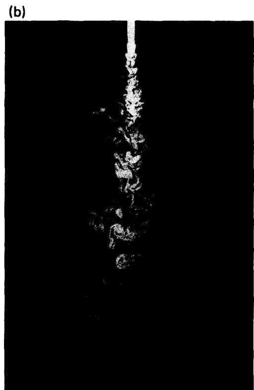
FIG. 5. Jet fluid field in the plane of symmetry of the jet ( Re = 2500 , d = 0.75 cm, 0 < x/d < 35 ). (a) Typical structure. (b) Evidence of spiral mode.
