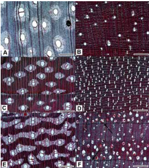
Figure 3–11. Transverse sections of various woods showing a range of hardwood axial parenchyma patterns. A, C, and E are woods with paratracheal types of parenchyma. A, vasicentric parenchyma in Enterolobium maximum ; note that two vessels in the middle of the view are connected by parenchyma, which is the feature also shown in E; the other vessels in the image present vasicentric parenchyma only. C, aliform parenchyma in Afzelia africana ; the parenchyma cells are the light-colored, thin-walled cells, and are easily visible. E, confluent parenchyma in Afzelia cuazensis . B, D, and F are woods with apotracheal types of parenchyma. B, diffuse-in-aggregate parenchyma in Dalbergia stevensonii . D, banded parenchyma in Micropholis guyanensis . F, marginal parenchyma in Juglans nigra ; in this case, the parenchyma cells are darker in color, and they delimit the growth rings (arrows). Scale bars = 780\ \mu\text{m} .
