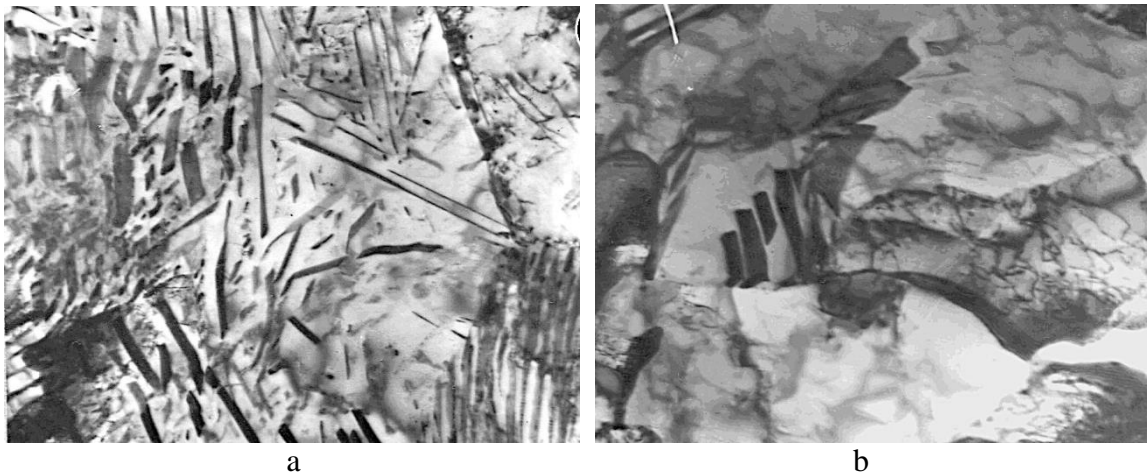
Fig. 3. The microstructure of metal in the axial part of the disc (magnification: 12,000)
