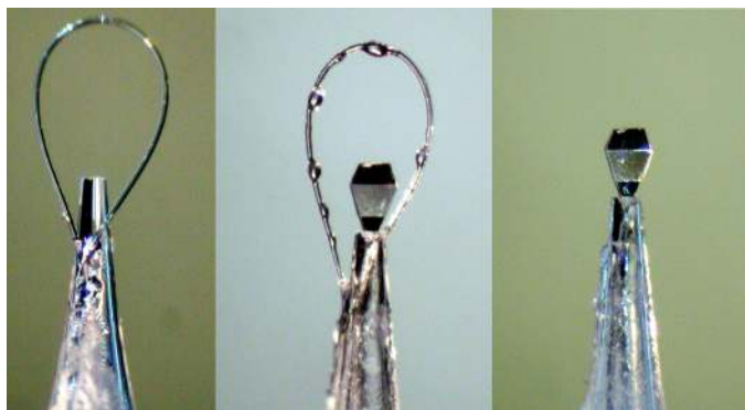
Figure 1 (a) A schematic illustration of the novel mounting technique. a. Picking up a protein crystal using nylon loop at the top of glass micropipette, and mounting the tools on the goniometer head intercepting the cryo-stream. b. Aspirating the cryo-buffer through the micropipette and flushing with the cold nitrogen stream. c. Removing the nylon-loop under cryo-conditions. (b) The mounting base for the novel mounting technique. This tool can hold the micropipette and aspirate the cryo-buffer through the flexible tube. (c) Left: The tip of the micropipette and nylon loop before picking up a protein crystal. The nylon loop was glued to the tip of the micropipette. Middle: The tip of the micropipette and a protein crystal after aspirating the cryo-buffer and freezing. Right: The tip of the micropipette and a protein crystal after removing the nylon loop. In the middle and right pictures, a thaumatin (SIGMA T-7638) crystal was used as the sample.
