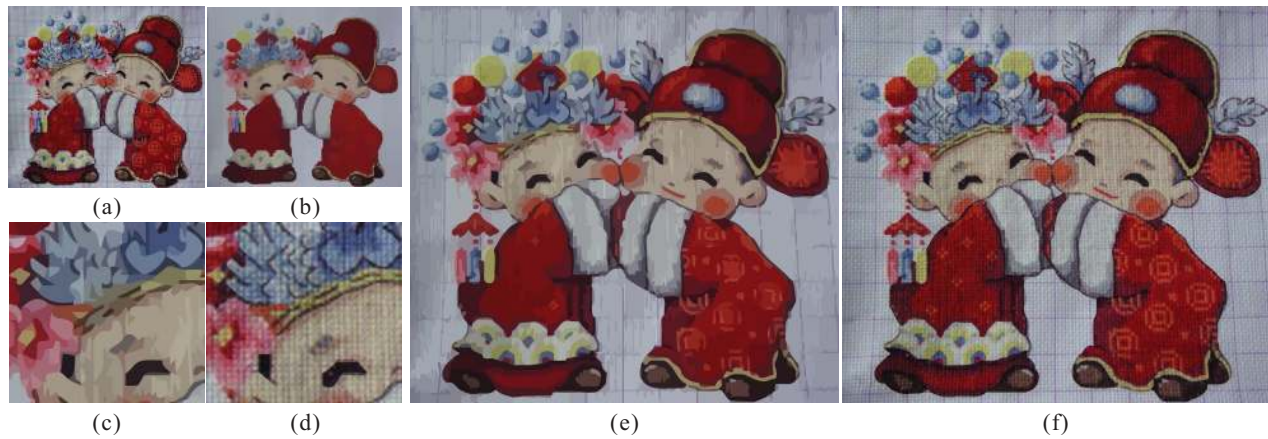
Figure 8: Structure vectorization. (a) Input. (b) Our structure image S . (e) Upscaled image after vectorizing (a) as a whole. (f) Upscaling result by only vectorizing (b) while the texture image is treated as a bitmap and is bilinearly interpolated. Close-ups of (e)-(f) are shown in (c)-(d).
