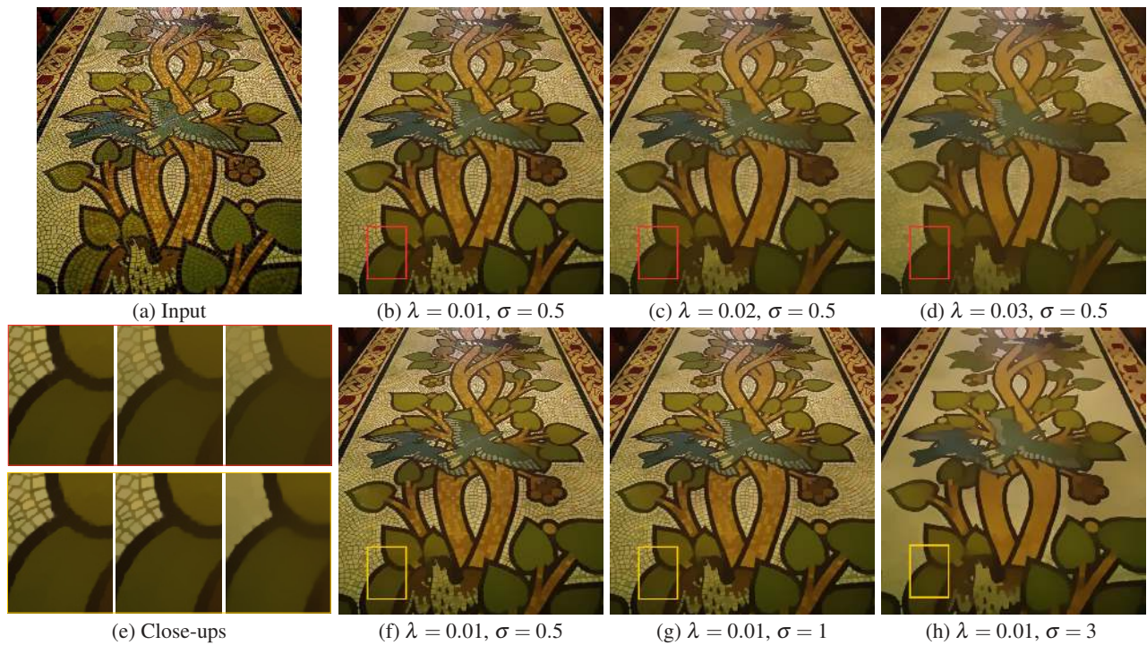
Figure 5: Effect of varying parameters. Tuning \sigma is much more effective than tweaking \lambda in structure-texture separation. (b)-(d) shows that varying \lambda blurs edges and cannot remove texture very well. In (f)-(h), we alter scale \sigma , which maintains sharp edges while separating texture.
