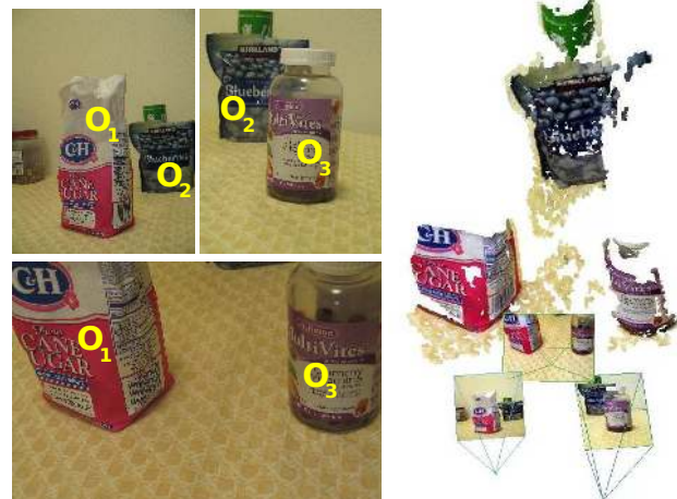
Figure 1. There are 3 objects in the scene: sugar ( O_1 ), blueberries ( O_2 ) and vitamin ( O_3 ). Each of the three images on the left can see only two out of the three objects, where the lack of three-view overlap prohibits standard resection. Note there are not reliable feature matches on the table due to the repeating patterns. The right image shows the dense reconstruction [3] from our reconstructed cameras using structure-less resection.
