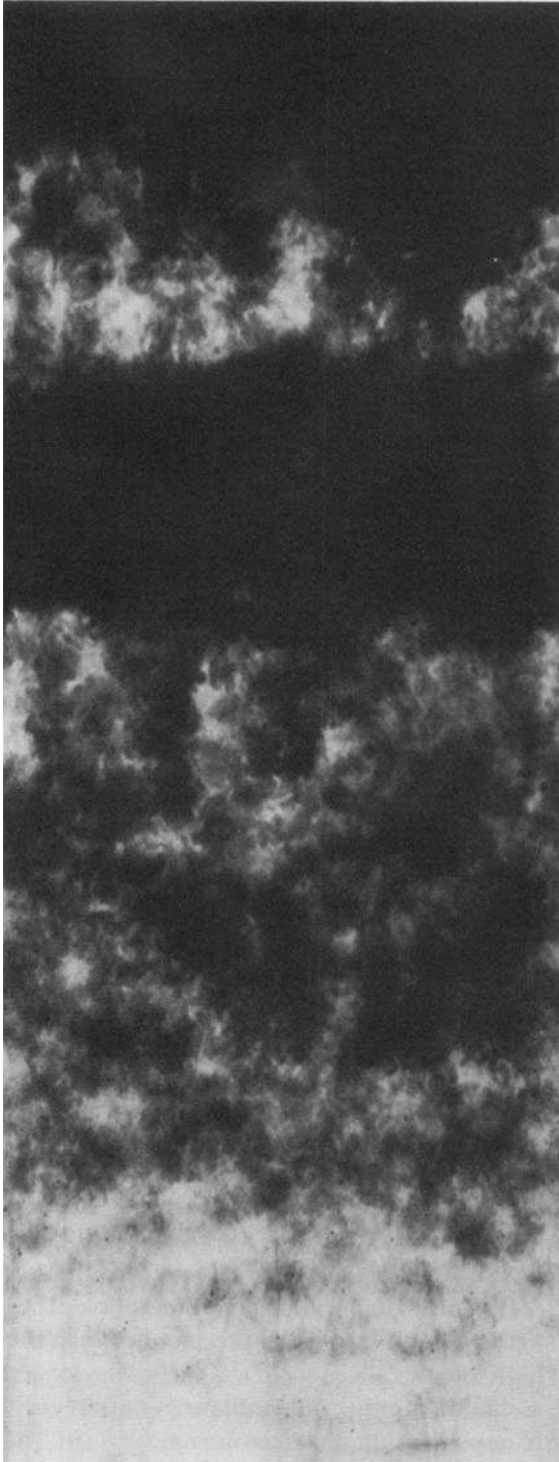
FIGURE 10. Plan view of the shear layer at U_1 = 96 \text{ cm s}^{-1} , r = 0.37 .
