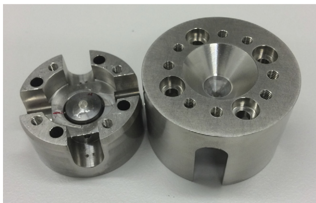
Figure 6. Typical DAC high-pressure apparatus with a large conical angular aperture.
