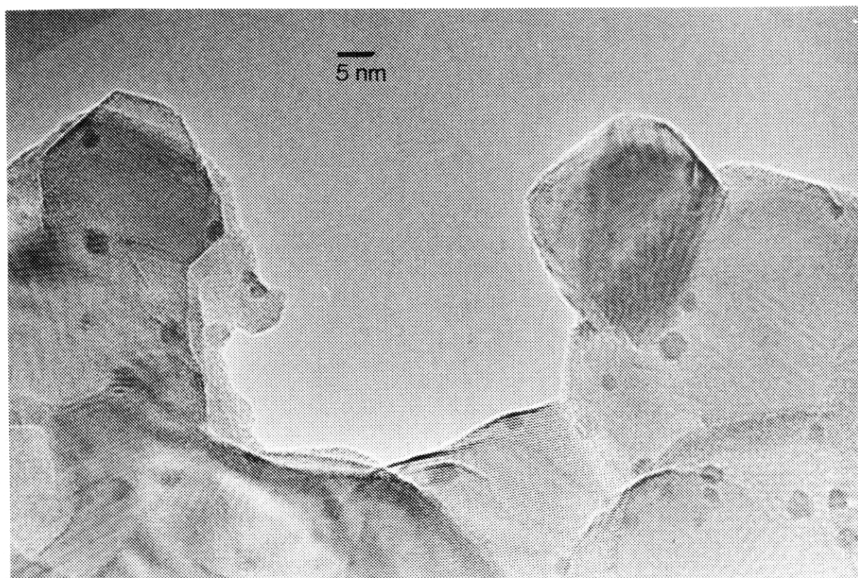
Figure 6. HRTEM micrograph of the Rh/TiO 2 catalyst after reduction at 773 K and subsequent passivation and in situ sintering.
