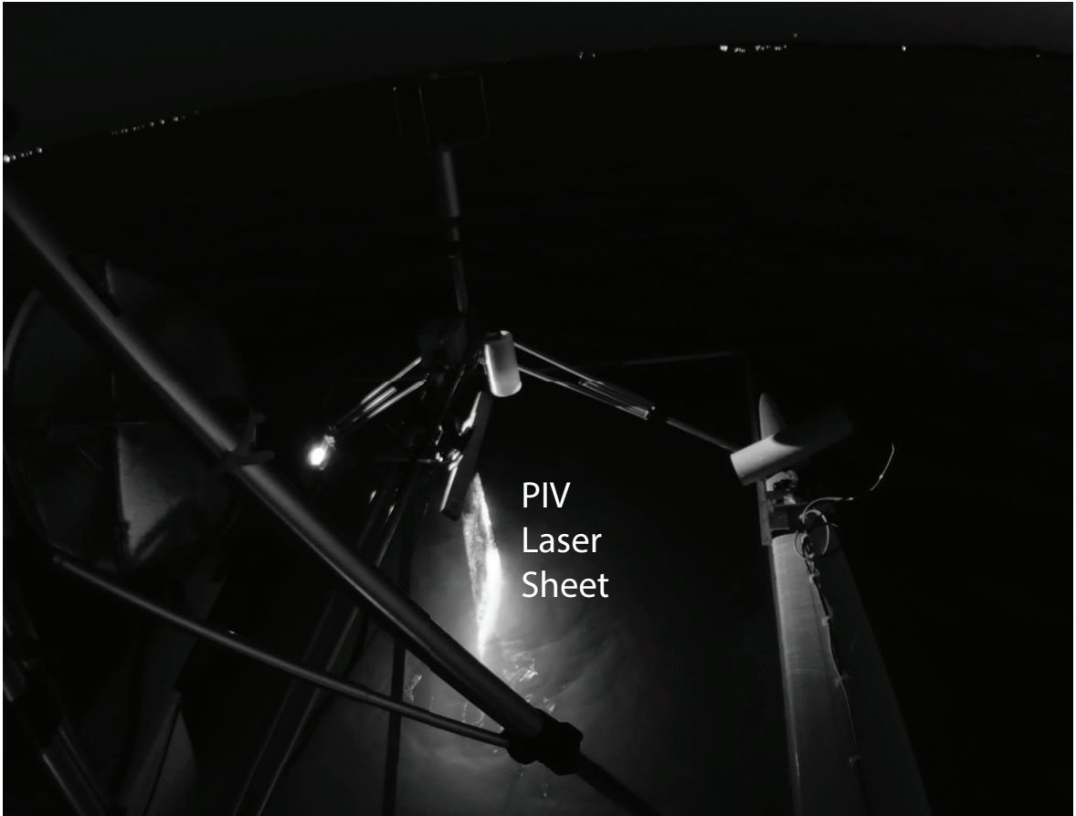
Figure B.3: Night time acquisition of PIV data in the incoming airflow above incoming waves, off the bow of Cheval Blanc .
