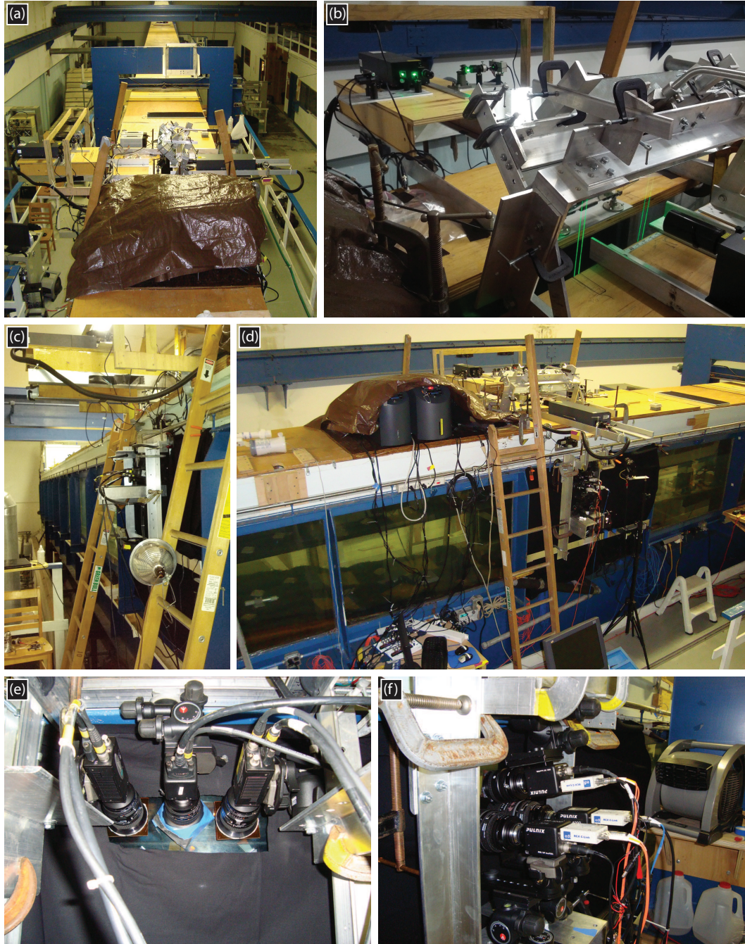
Figure 2.3: Photos of the imaging system, capable of measuring simultaneously airflow velocities up to 100 \mu\text{m} away from the water surface (2D PIV/PIVSD), spatial wave profiles (LFV), and water height time series (WG). (a) Downwind top view of the system, positioned 22.7 m downwind of the wind input. (b) Right top view of the system, with the 2 pairs of continuous WG laser beams (green), located respectively upwind and downwind of the PIV imaging section. (c) Left downwind view of the LFV and WG camera and LFV laser setup. (d) Right downwind view of the system. (e) WG and LFV cameras. (f) PIV and PIVSD cameras.
