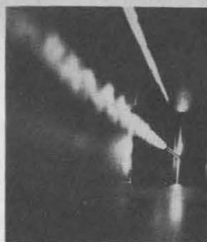
Fig. 13 View upstream in a wind tunnel of a coflowing jet with plane of symmetry illuminated by a vertical sheet of light. Jet diameter d = 1 in.; U_j/U_\infty = 1.5 ; U_j d/\nu = 3500 ; x/d = 80 .
