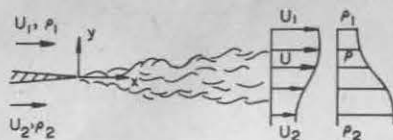
Fig. 1 Plane mixing layer between two streams with velocities U_1 and U_2 , densities \rho_1 and \rho_2 .
