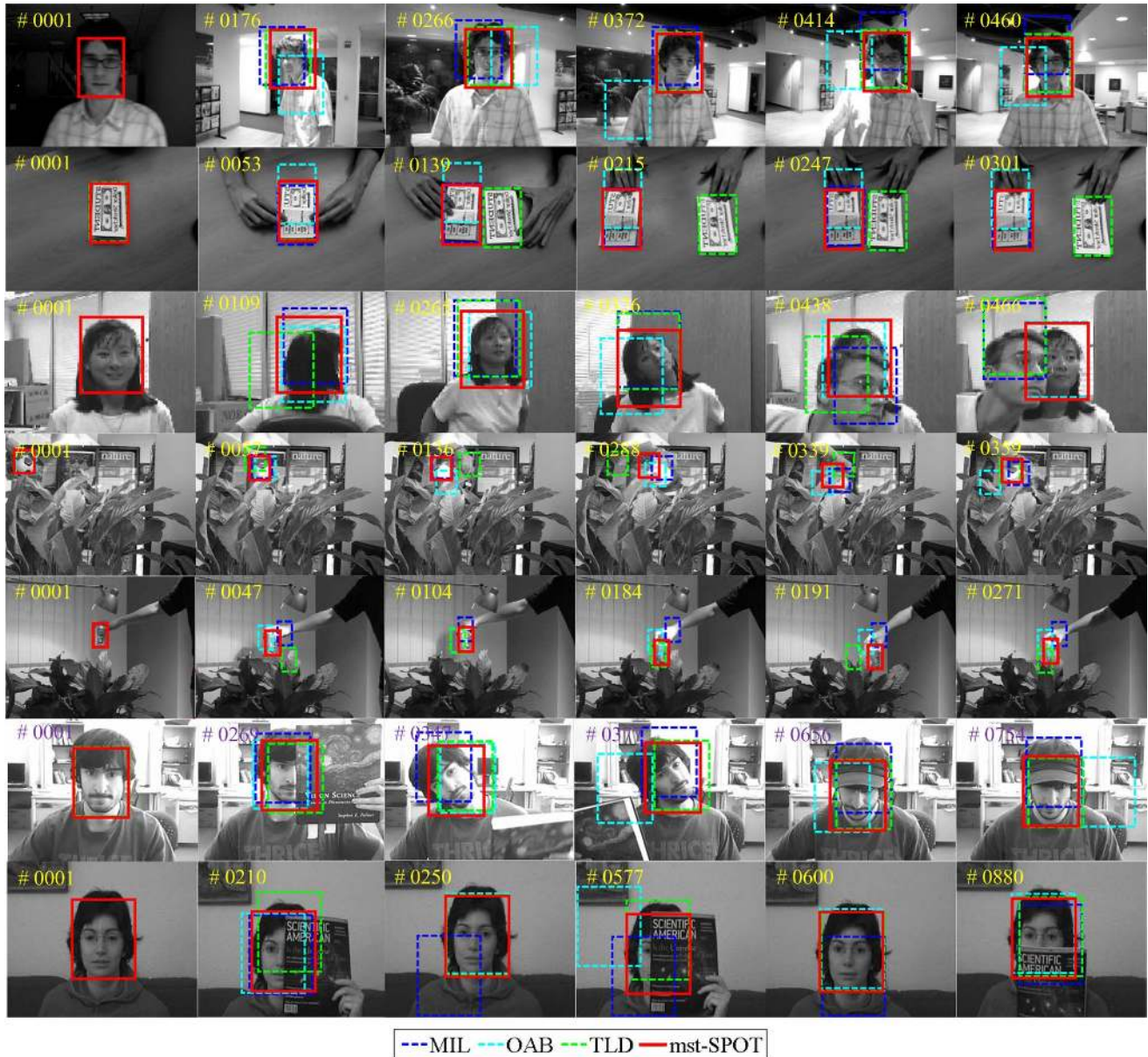
Figure 2. Tracking results on seven of the twelve videos ( David Indoor , Dollar , Girl , Tiger 2 , Coke Can , Occl. Face 2 , and Occl. Face ) obtained by the MIL, OAB, TLD, and mst-SPOT trackers. Figure best viewed in color.
