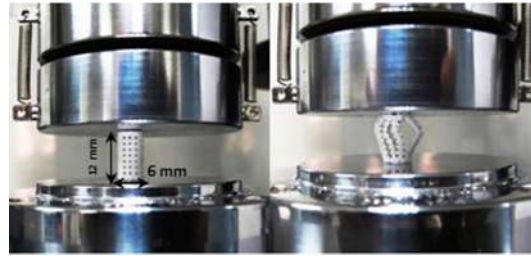
Fig 22. Specimens under compression test.
