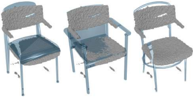
Figure 3: Rough alignment of repository models with input scan.
