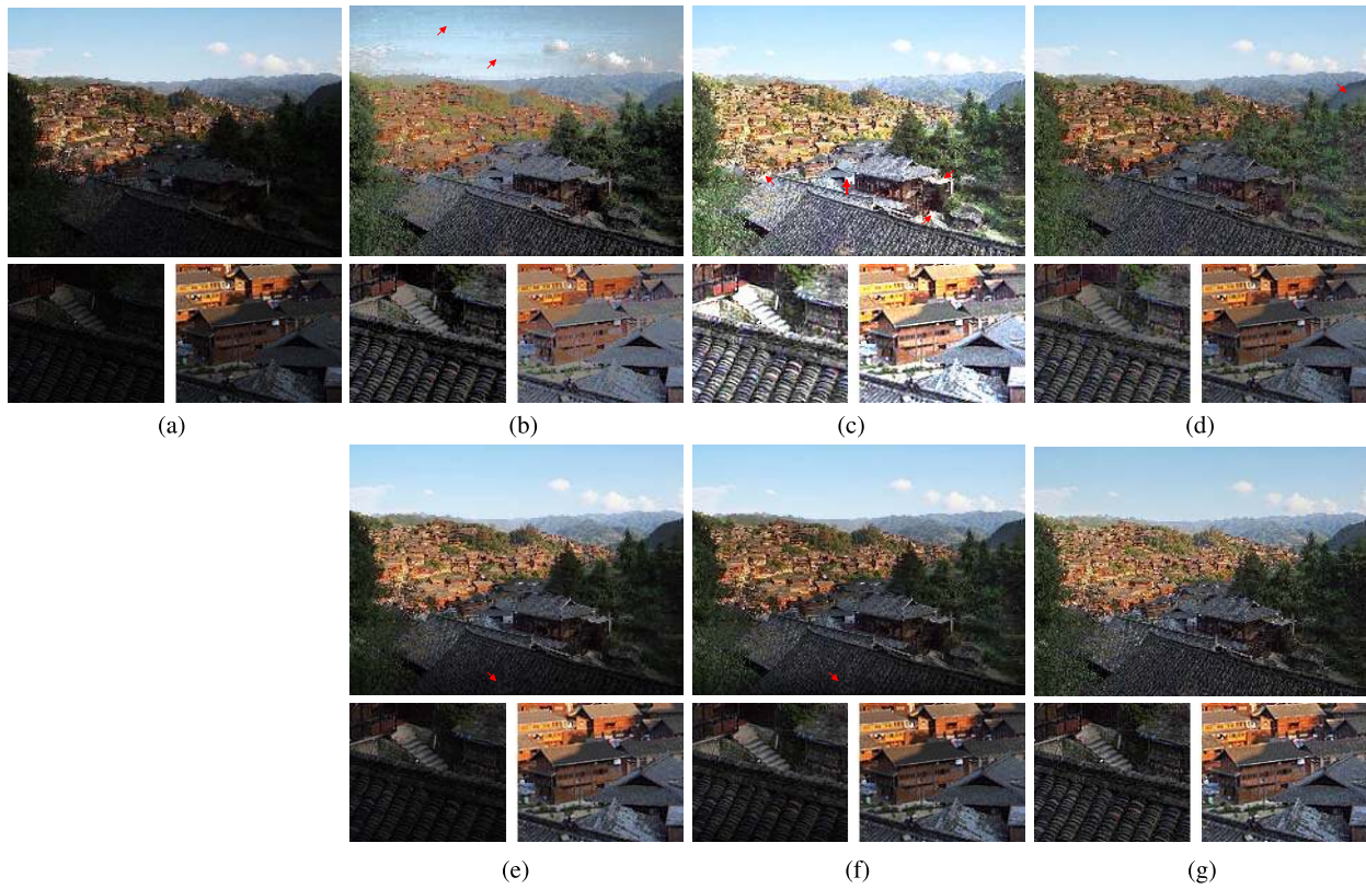
Fig. 5. Comparisons of low-light image enhancement results for test image #18. Red arrows indicate artifacts or degradation. (a) Input. (b) HE. (c) LIME [13]. (d) NPE [11]. (e) PIE [23]. (f) SRIE [14]. (g) Proposed with model (3).
