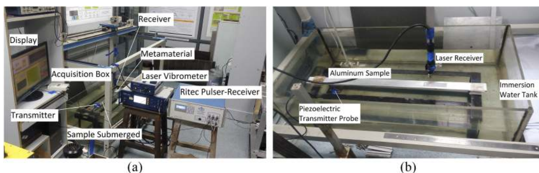
FIG. 3. Photograph of the (a) experimental setup and (b) transmitter, sample, and receiver position.
