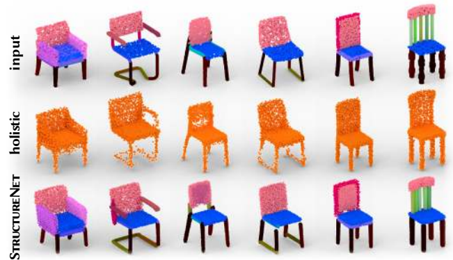
Fig. 8. Reconstruction compared to a holistic approach. We reconstruct the point cloud representation of the shapes in the top row with a holistic approach (orange) that does not use structure, and compare to STRUCTURENET. The holistic approach suffers from noise that results in a loss of detail, whereas reconstruction errors in our approach take the form of slightly modified chair structures, such as the hole added to the backrest in the third column. However, the functional realism of the shape is usually preserved and the explicit structure allows us to preserve significantly more detail.
