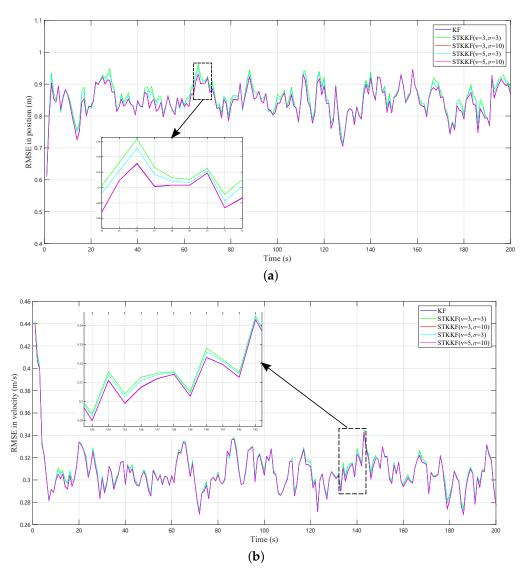
**Figure 1.** RMSE results of KF and STKKF in case 1 where RMSE is taken over 100 Monte Carlo simulations: (**a**) position. (**b**) velocity.
