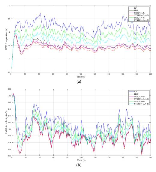
**Figure 2.** RMSE results of different filters in case 2 where RMSE is taken over 100 Monte Carlo simulations: (a) position. (b) velocity.
