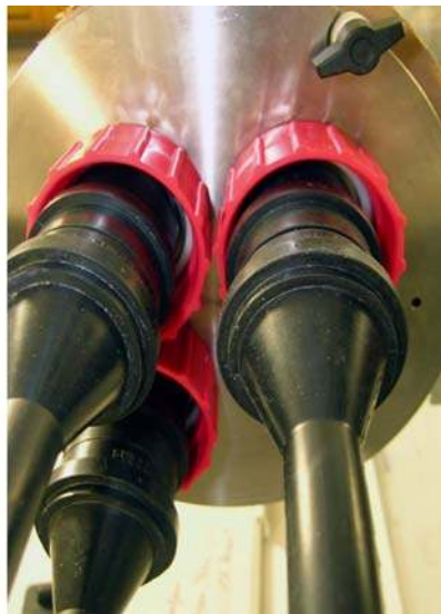
Fig. 3. View of the lower flange of an electronics container showing the three connections to the optical module spheres plugged into the SubConn® bulkhead connectors.
