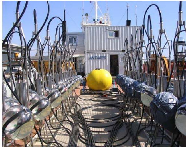
Fig. 6. The full scale mechanical prototype line on the deck of the deployment ship, showing the simulated optical modules, flotation buoy and the inter-storey sections of electro-mechanical cable
