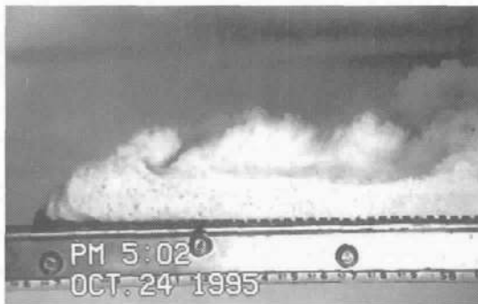
Fig. 2: Head of a subaqueous debris flow and overlying suspended-sediment cloud simulated within the flume at St. Anthony Falls Laboratory of the University of Minnesota. Note how the head of the debris flow is overriding the wedge of water in front of it and has detached from the grooved, dark-colored flume bed. This greatly reduces the bed friction that would otherwise retard the movement of the debris flow, allowing it to travel much farther downslope than it would under subaerial conditions. Image length is 49 cm.
