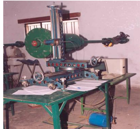
Figure 5. A view of the free jet facility
