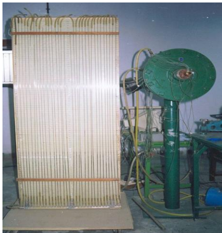
Figure 4. Jet facility with the control chamber and multi-tube manometer
