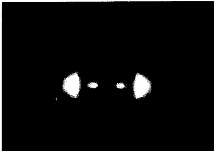
Fig. 12. WAXS pattern of a quenched sample of 60-mole % PHB/PET system subjected to extensional flow at \dot{\epsilon} = 2.5 \text{ sec}^{-1} and a temperature of 275°C. Flow direction is along the vertical axis.
