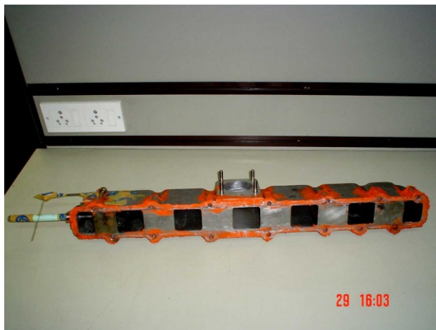
Figure 1. Experimental swirl plate set up for 2-valve port variable swirl mechanism (color image see on our web site)
