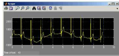
Fig. 3. This simulink Scope shows an acquired ECG signal with a sampling frequency of 1200 Hz
