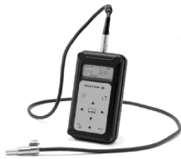
Fig.1.Noise Dose Meter 4444 used for this study
