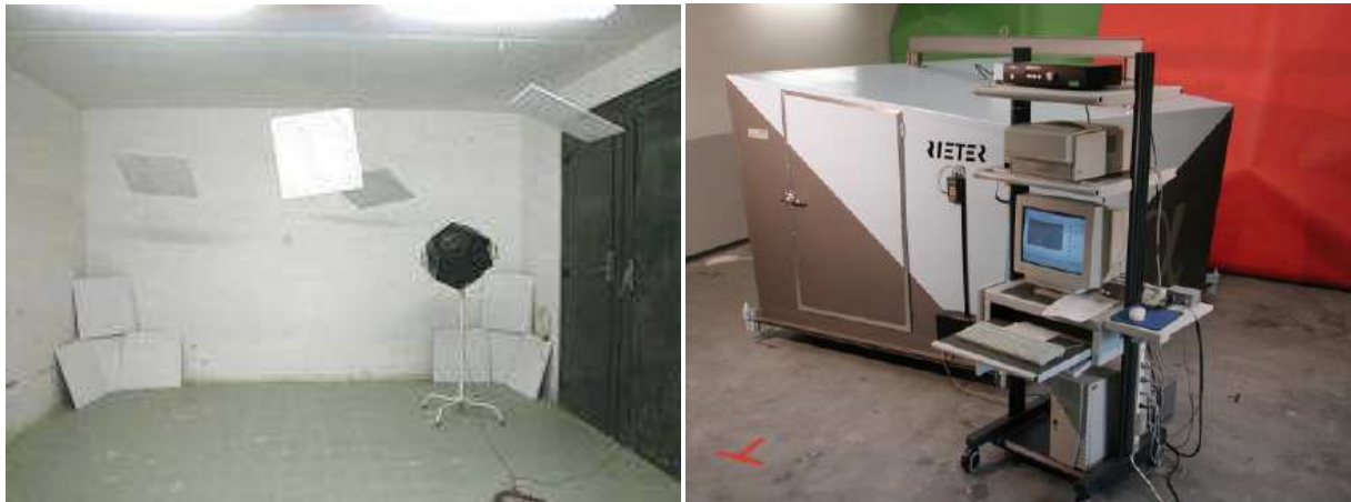
Fig. 2-6. Two examples of reverberant rooms. Left: large room with omni-directional sound source and deflectors, source [42]. Right: Alpha cabin, source [40].
