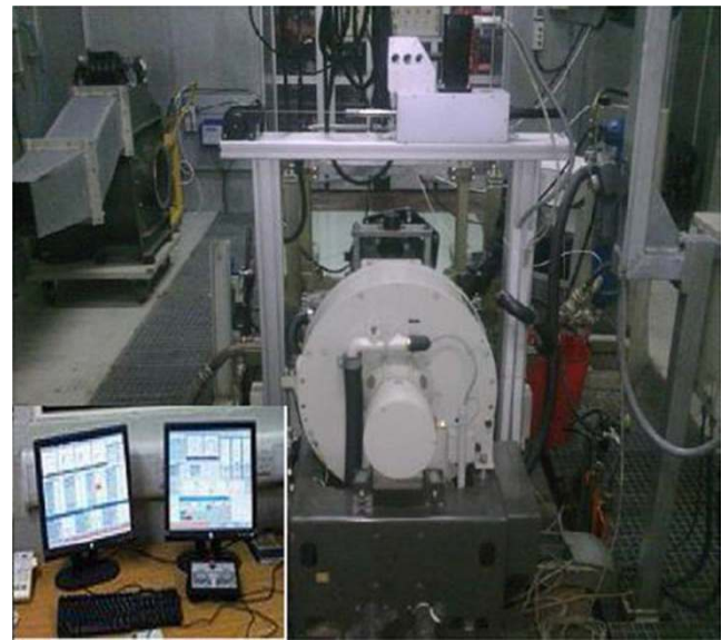
Fig. 1 Control panel and test engine on dynamometer
