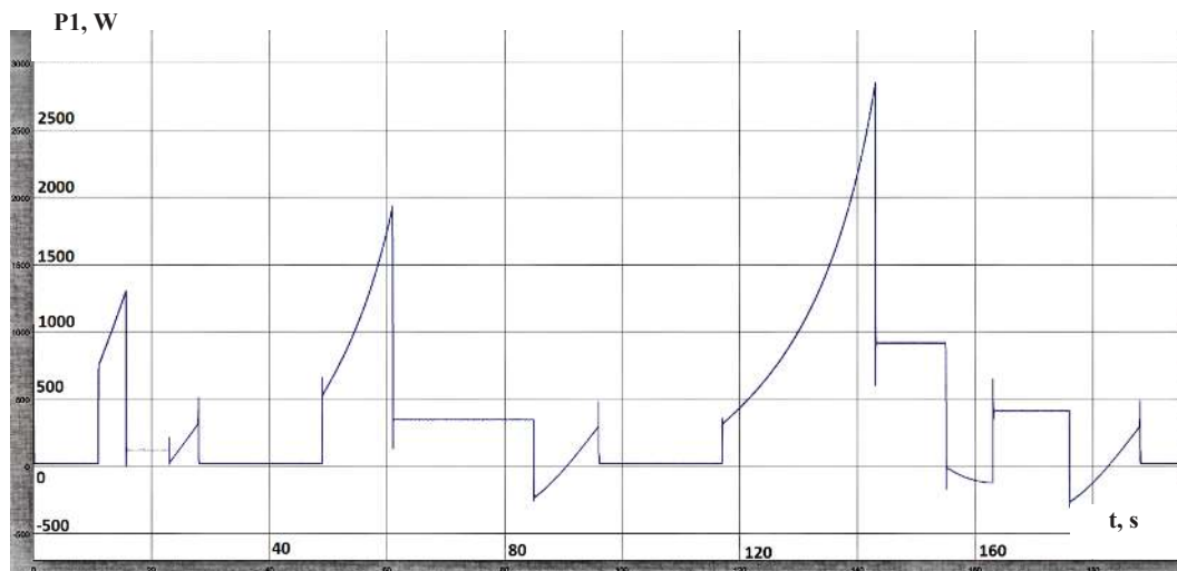
Fig. 3. Time dependence of power consumed by the electric scooter, powered by a source without ultracapacitor
