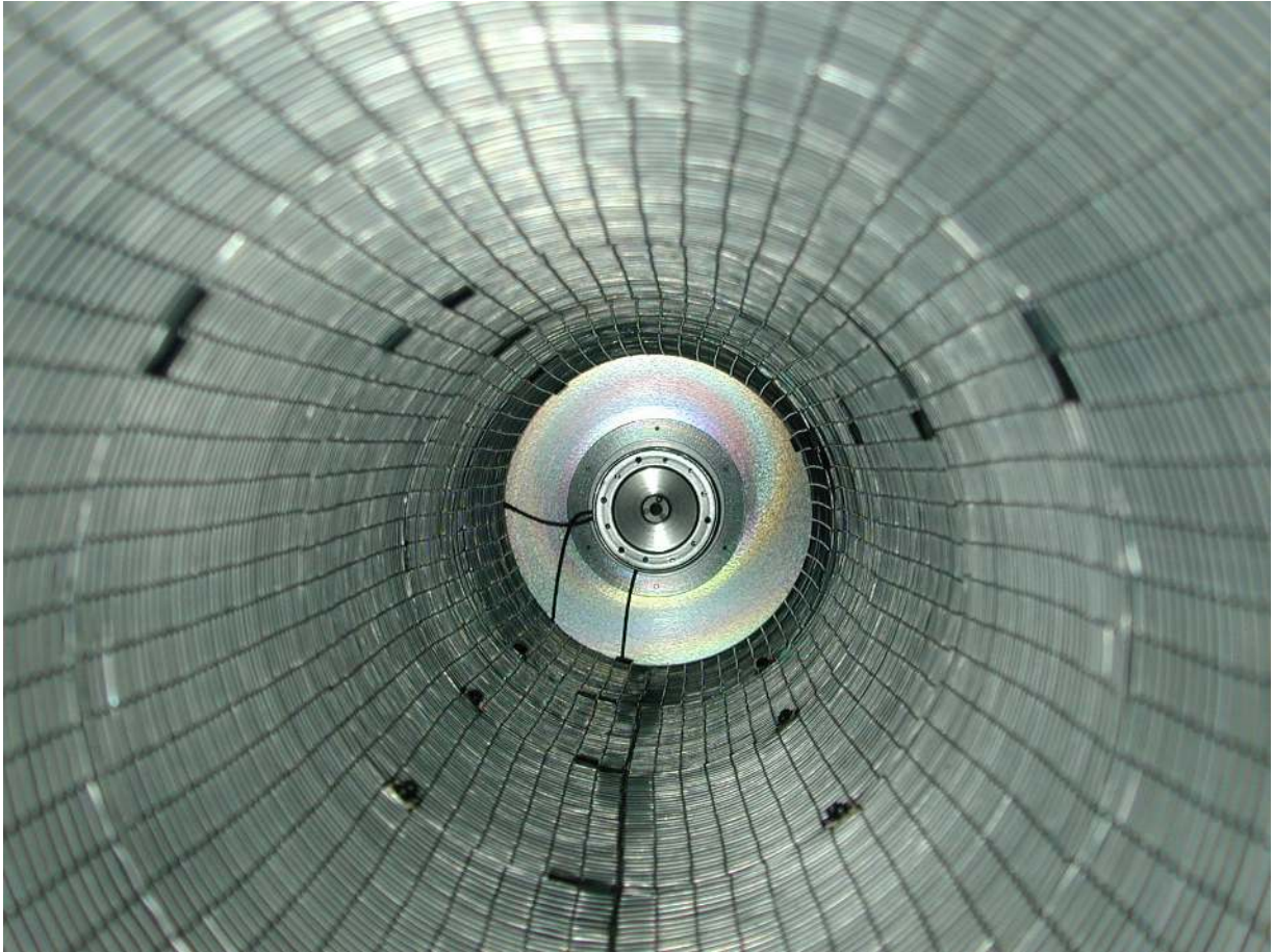
Figure 18: A cylindrical metal mesh inside the beam pipe in the magnetic final focus section.
